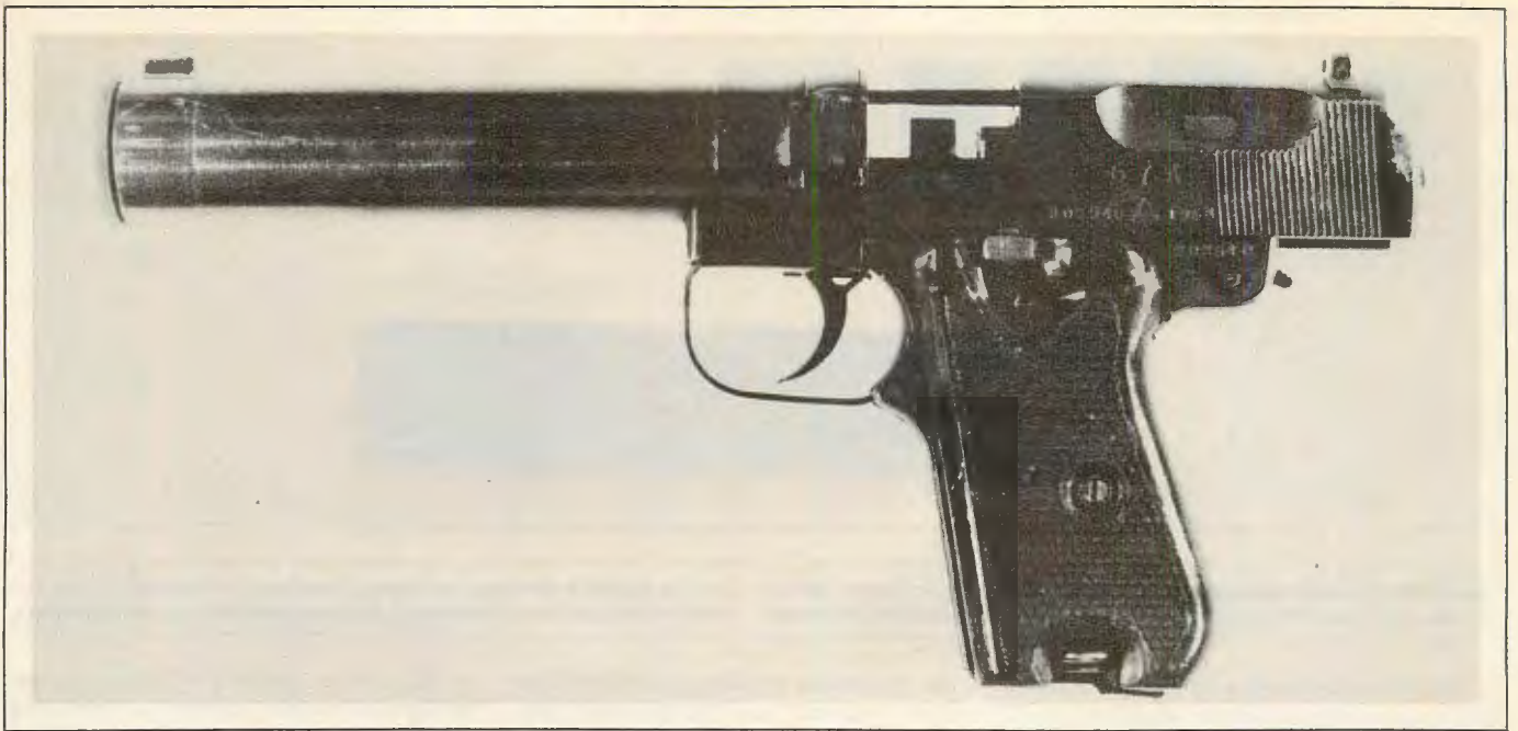
With receiver back, model 67 shows lineage of model 64. Pistol weighs 20 ounces and is 8.9 inches long.
